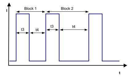
Block1: special locked rotor protection: 5 cycles t3 / t4 = 0,6 s / 1 s Block2: locked rotor protection t3 / t4 = 0,6 s / 10 s
